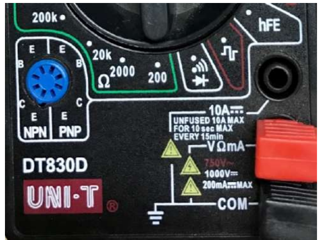
Figure 141: Connect test cables
