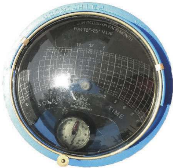
Figure 57: Dome shaped cover of solar pathfinder for shadow analysis
