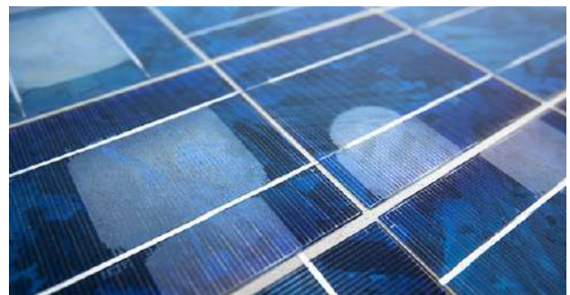
Figure 34: Tiny Hairline Cracks
